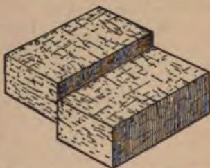
FIG. 55.—A fault of vertical displacement.
